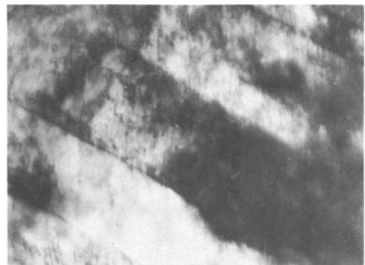
Figure 2 Thin-foil electron micrograph of Fe–1.31% As alloy, showing array of laths. Within the laths high densities of tangled dislocations (cell walls) can be resolved,  $\times 40\,000$ .
