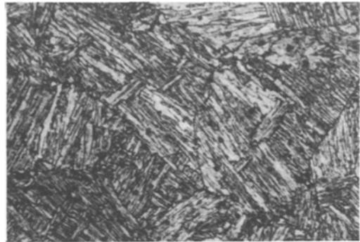
Figure 1 Light micrograph showing lath martensite in an iced brine quenched Fe–1.31% As alloy. Etched with 1 g picric acid, 10 ml hydrochloric acid and 10 ml nitric acid in 50 ml ethanol,  $\times 740$ .
