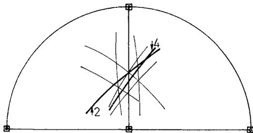
Figure 5 Trace analyses of normals to lath boundaries showing that habit plane of martensitic lath is close to  $\{110\}_{\alpha}$  (numbers indicate coincident traces).
