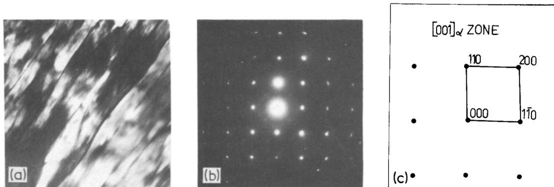
Figure 3 Small-angle laths in quenched Fe-0.85% As alloy. (a) Thin-foil micrograph,  $\times 20\,000$ ; (b) diffraction pattern; (c) analysis of diffraction pattern.
